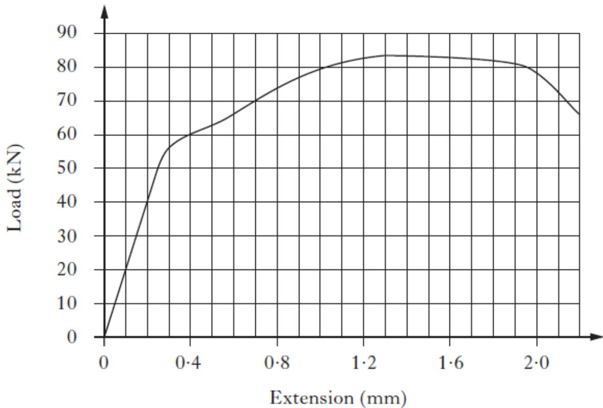
The test specimen was 120 mm long with a rectangular cross-section of 26 mm  $\times$  6 mm.
