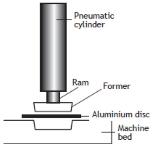
Aluminium alloy is a ductile material.
