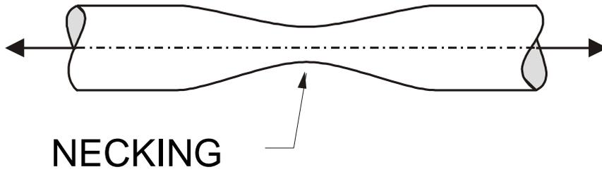
'Necking' reduces the cross-sectional area of the specimen, which in turn reduces the strength of the sample. The sample eventually reaches point 'D' where it breaks or fractures. This is known as the **breaking point**. The shape of a typical fractured specimen is shown below.
