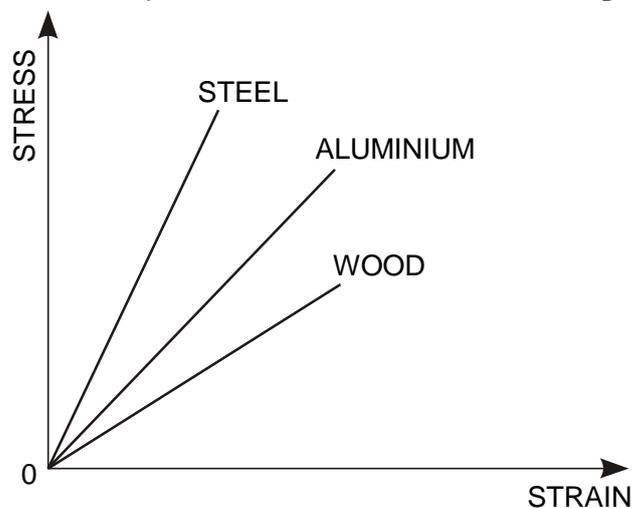
We also find that within the elastic limit, the graphs are a straight line therefore conforming to Hooke's Law. This means that stress is proportional to strain. We use the principle of Hooke's Law to find a value called young's Modulus. Young's Modulus is sometimes called the Modulus of elasticity and is calculated using the formula:
