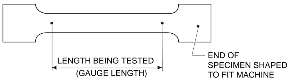
The principle of tensile testing is very simple. As the force is applied to the specimen, the material begins to stretch or extend. The tensometer applies the force at a constant rate and readings of force and extension are noted until the specimen finally breaks. These readings can be plotted on a graph to show the overall performance of the material.
