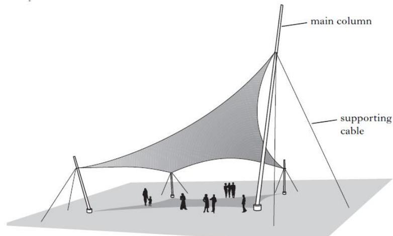
The supporting cables have an effective diameter of 10 mm and the safe working strain is 0.0009.
