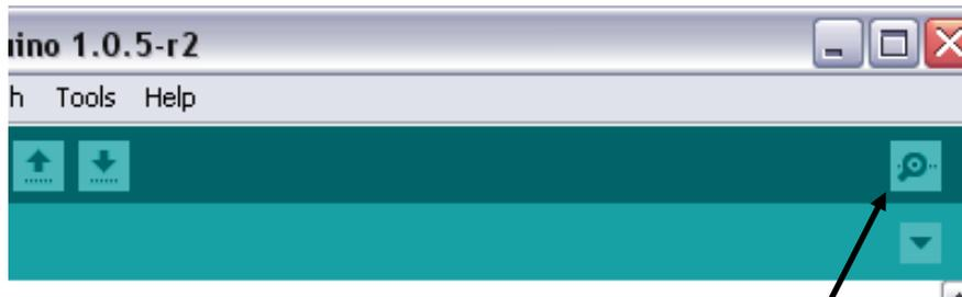
When it has uploaded I can press the Serial monitor button, which opens a new dialogue box and "prints" what I put in the serial print boxes once it has completed
